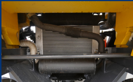
03 The combined radiator with serpentine wave and optimized heat dissipation channel enhance the heat dissipation capability to keep engine reliability even in heavy-duty applications.
