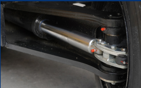
02 Heavy duty steering axle with tapered bearings.
